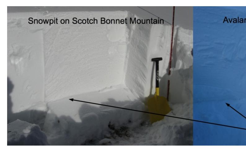
The photo on the right is from a snowmobile triggered avalanche on Crown Butte on 11-26. The photo on the left shows a nearly identical snowpack on nearby Scotch Bonnet Mtn the same day where a stability test broke on facets near the ground (ECTP 17). A similar layer of facets produced the human triggered avalanche on Crown Butte. Slopes with recent avalanches are clear evidence that similar slopes with a similar snowpack structure are prime places to trigger more avalanches. Photo: GNFAC
