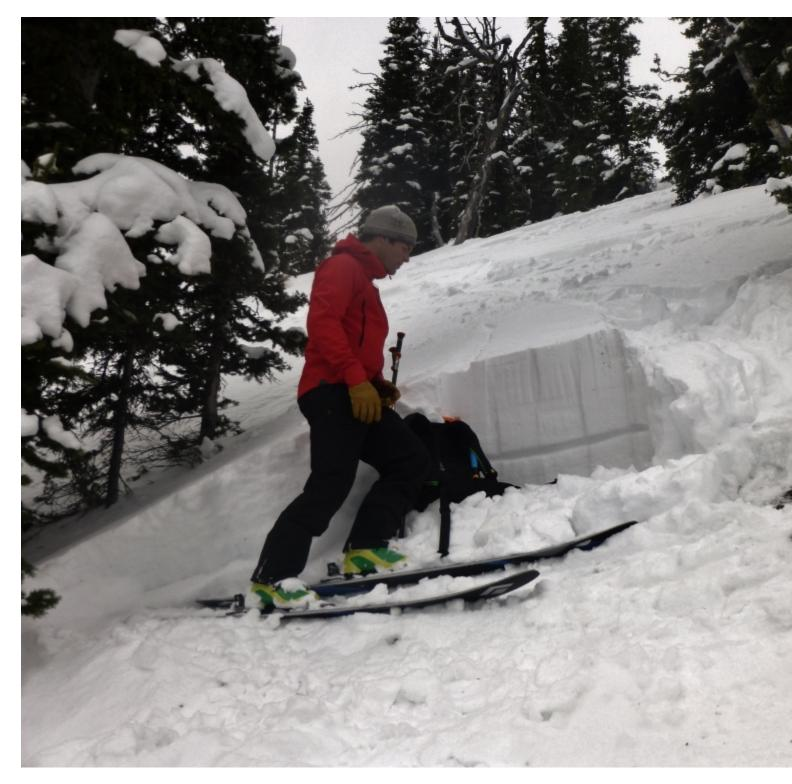
This photo shows where the skier's tracks entered the avalanche and approximately where he triggered it. The weak layer of facets that fractured can be seen scooped out of the snow. The crown profile can be seen here: http://www.mtavalanche.com/images/13/ellis-crown-profile?size=\_original Photo: GNFAC
