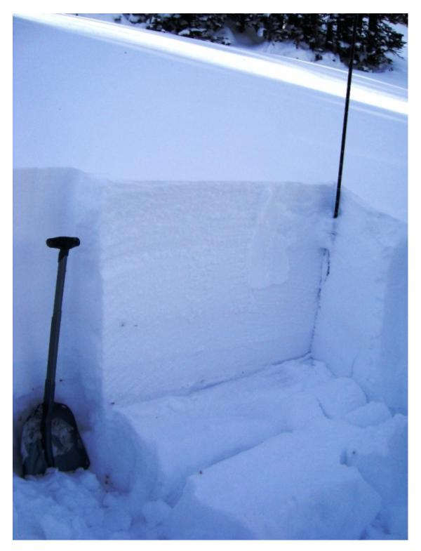
This 115cm deep pit was dug on an east aspect at 9,100 feet near Hyalite Lake. The ECT failed on 21 taps, twice, and broke clean indicating unstable conditions. It is breaking on 5 cm of sugary facets sitting on an ice crust. Cracking, collapsing and avalanches were seen on this layer in the last 48 hours. Photo: GNFAC
