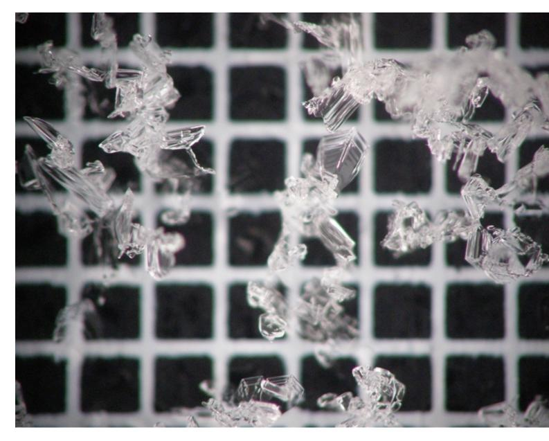
These facets may be a future weak layer. They form when solar radiation heats upper layers of the snowpack, but the surface of the snowpack emits long wave radiation to a clear sky and remains cool resutling in a strong temperature gradient. Photo: YCSP
