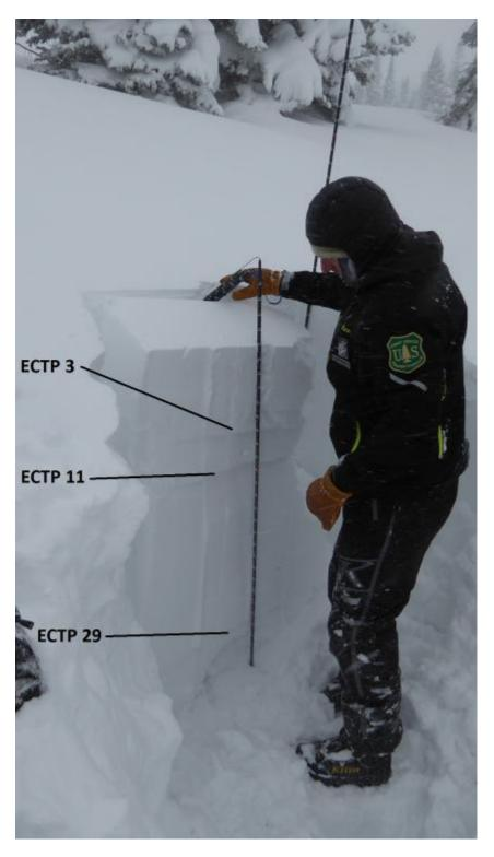
Dave Zinn of the GNFAC gets 3 layers breaking in his Extended Column Test. About 3 feet of snow fell in the last 4 days which got blown into wind slabs. The weight of the new snow is also creating instability on a weak layer of sugary facets near the ground. Photo: GNFAC
